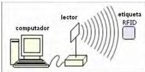
Figure 1: Components of an RFID system. Source: Courtesy of GS1 /Peru.
